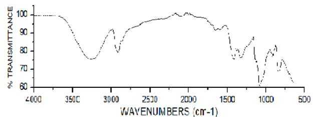
**Figure 1 (a). FT-IR spectra of 0.3 mg Gamma alumina-PVA membrane**
