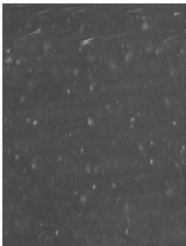
Figure 2 (a) . SEM images of the top view of the synthesized membranes: 0.3 mg Gamma alumina-PVA membrane ( $\times 1200$ )
